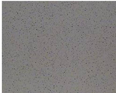
Photomicrograph of Tecsic-P Silicon Carbide (200x).
