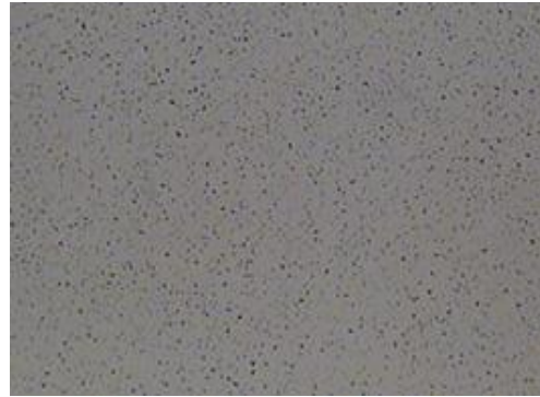
Photomicrograph of Tecsic-P Silicon Carbide (200x).
