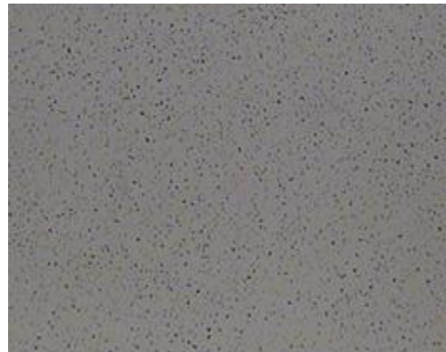
Photomicrograph of Tescic-P Silicon Carbide (200x).
